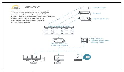
Figure 2: VMware and IGEL Architecture
