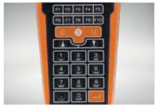
Membrane keypad with 10 function keys
